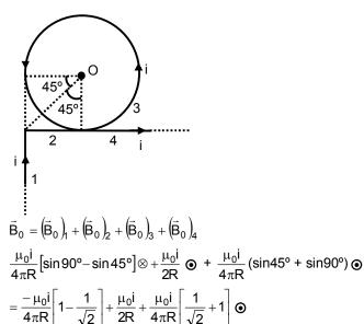
$$=\frac{\mu_0 i}{4\pi R} \left[-1+\frac{1}{\sqrt{2}}+2\pi+\frac{1}{\sqrt{2}}+1\right] \boldsymbol{\odot} \\ \qquad =\frac{\mu_0 i}{4\pi R} \left[\sqrt{2}+2\pi\right] \boldsymbol{\odot} \\ \qquad =\frac{\mu_0 i}{2\pi R} \left[\frac{1}{\sqrt{2}}+\pi\right] \boldsymbol{\odot}$$
