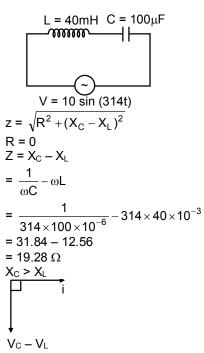
$$\begin{split} i &= \frac{V_0}{Z} sin \bigg( 314t + \frac{\pi}{2} \bigg) \\ \therefore \qquad i &= \frac{V_0}{Z} cos(314t) \qquad \Rightarrow \qquad i = \frac{10}{19.28} cos(314t) \qquad \Rightarrow \qquad i = 0.52 cos (314t) \end{split}$$
